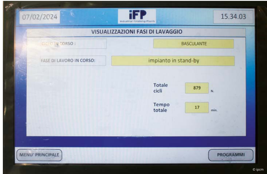
The control PLC connected to the company's MES management system and the PLC display for cleaning cycle management.
