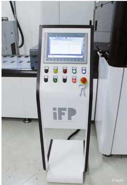
The control PLC connected to the company's MES management system and the PLC display for cleaning cycle management.
